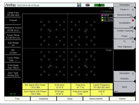
Figure 5-7. Constellation Measurement View
