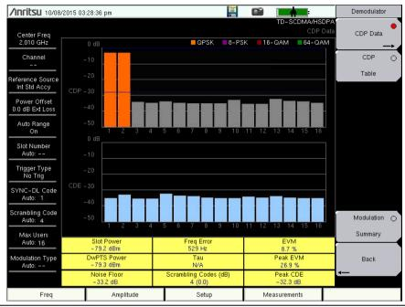
Figure 4-4. TD-SCDMA/HSPA+ Demodulator, CDP Data
