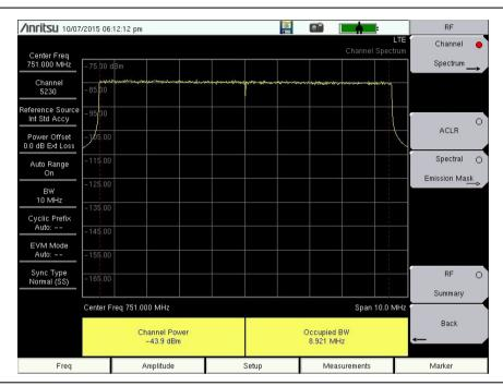
Figure 5-2. Channel Spectrum
