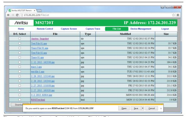
Figure 7-4. Web Remote Control Window - File List Tab
