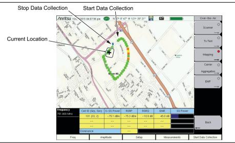
Figure 7-1. Outdoor Coverage Mapping (GPS On)
