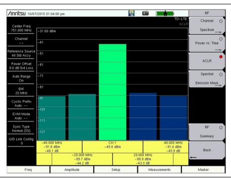
Figure 6-4. Adjacent Channel Leakage Ratio
