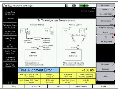
Figure 5-10. Tx Time Alignment
