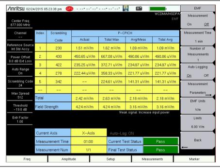
Figure 8-13. W-CDMA EMF Measurement Results
