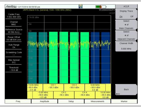
Figure 3-4. ACLR Multi-channel Measurement
