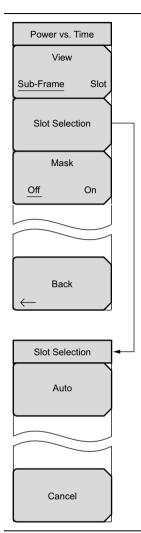
**View:** Press this submenu key to display the Power vs. Time graph in either the Sub-Frame view or the Slot view.
