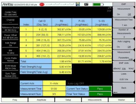
Figure 8-7. LTE EMF Measurement Results
