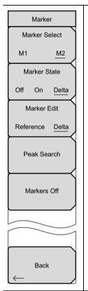
**Marker Select:** Selects the active marker M1 or M2. The underlined marker is active marker. Each press of the submenu key moves the underline to the other marker.
