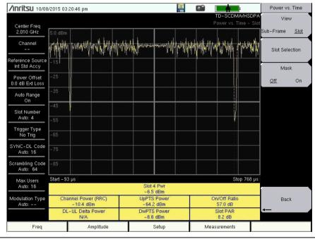
Figure 4-3. TD-SCDMA/HSPA+ Power vs. Time: Slot Measurement
