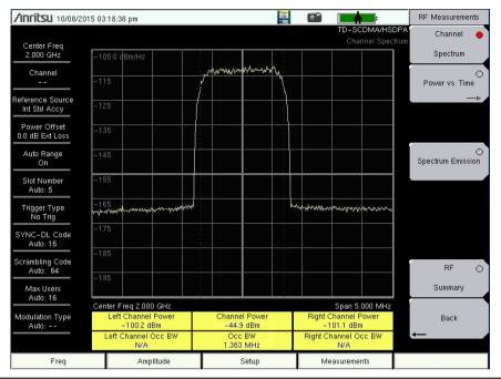
Figure 4-1. TD-SCDMA/HSPA+ Channel Spectrum
