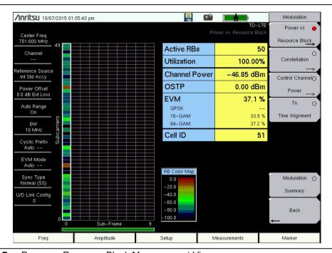
Figure 6-7. Power vs Resource Block Measurement View
