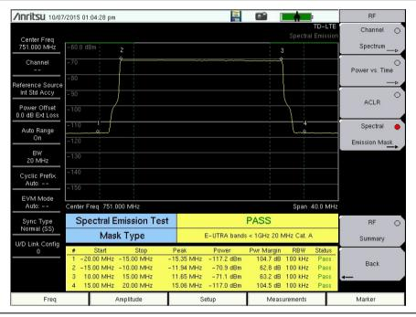
Figure 6-5. Spectral Emission Mask
