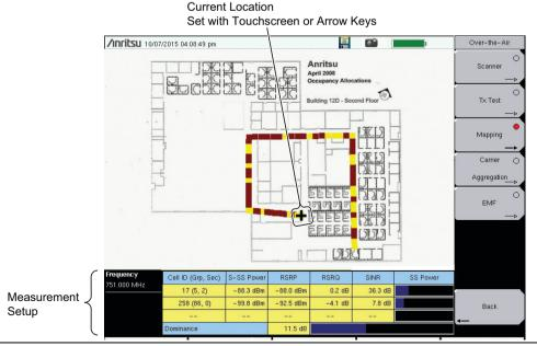
Figure 7-2. Indoor Coverage Mapping (GPS Off)
