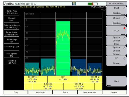
Figure 3-3. ACLR Measurement
