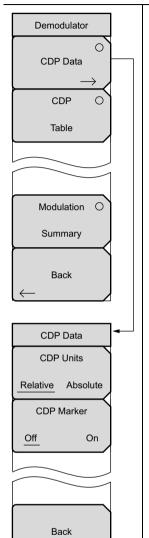
**CDP Data:** Press this submenu key once to activate this test. Press this submenu key again to display the CDP Data menu and further set up the measurement.
