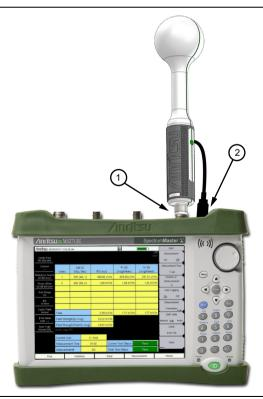
Figure 8-1. Connecting the Anritsu Isotropic Antenna
