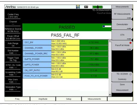
Figure 4-7. TD-SCDMA/HSPA+ Pass/Fail Measurements
