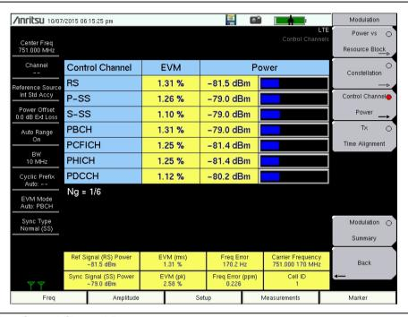
Figure 5-8. Control Channel Power
