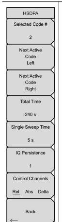
**Selected Code:** Press this submenu key to select the active code, using the arrow keys, rotary knob, or numeric keypad. The range is 0 to 255 or 0 to 511 depending on the Max Spreading Factor set under the Setup main menu. Refer to "Setup 1/2 Menu" on page 3-28.
