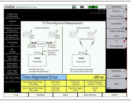
Figure 6-10. Tx Time Alignment
