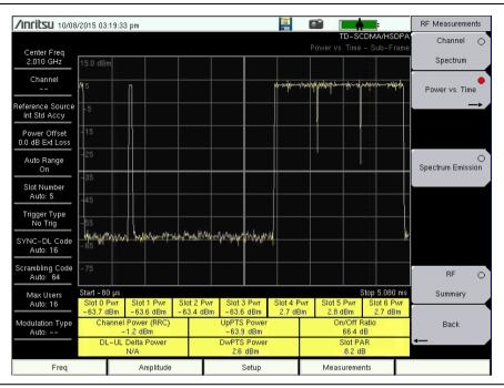
Figure 4-2. TD-SCDMA/HSPA+ Power vs. Time: Sub-Frame Measurement
