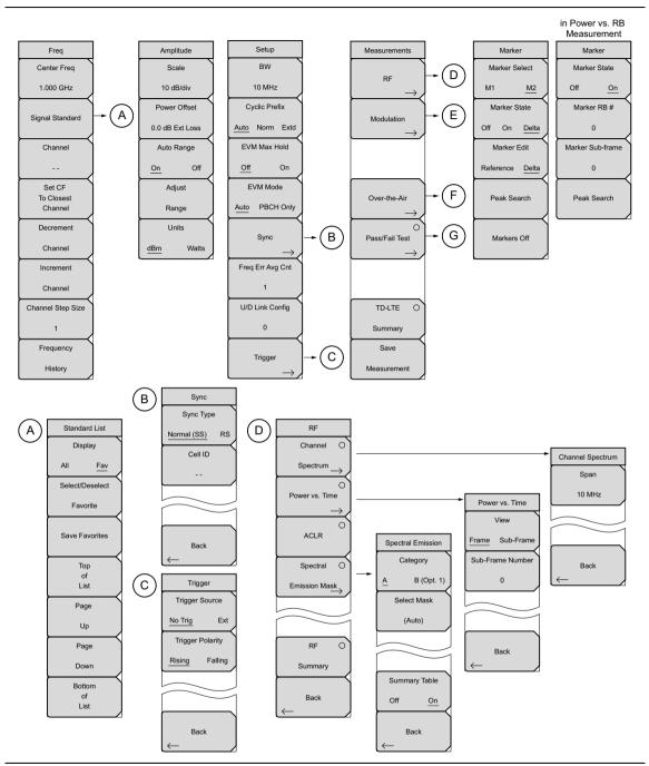
Figure 6-16. TD-LTE Menu Layout (1 of 3)
