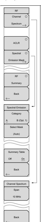
**Channel Spectrum:** Displays the spectrum of the input signal. Beneath the graph, values for the following measurements are displayed: Channel Power and Occupied BW. Channel Power is displayed in dBm or Watts (based on the Units submenu setting in the **Amplitude** menu) and Occupied BW is displayed in MHz. Press this button again to list the Channel Spectrum menu to set the Span.
