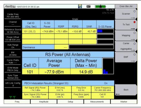
Figure 6-13. Over-the-Air Tx Test Measurement
