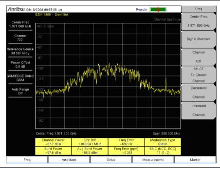
Figure 2-1. GSM Single Channel Measurement
