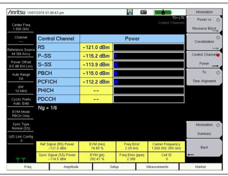
Figure 6-9. Control Channel Power
