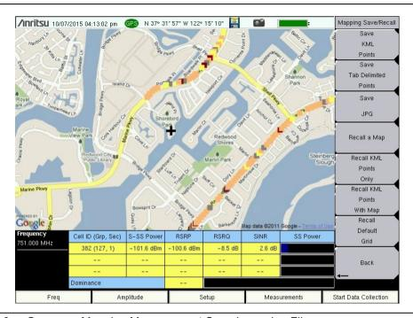
Figure 7-6. Coverage Mapping Measurement Saved as a .jpg File
