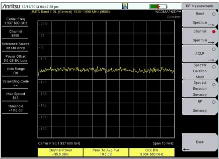
Figure 3-2. Channel Spectrum
