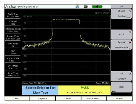
Figure 5-4. Spectral Emission Mask
