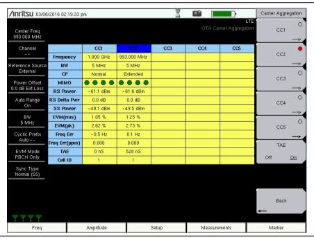
Figure 5-14. Over-the-Air Carrier Aggregation Measurement
