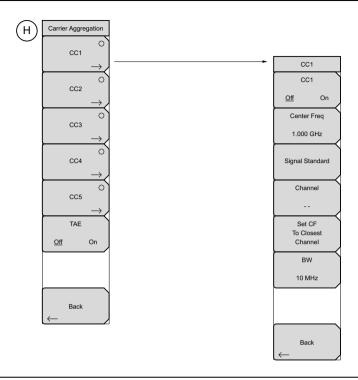
Figure 6-18. TD-LTE Menu Layout (3 of 3)
